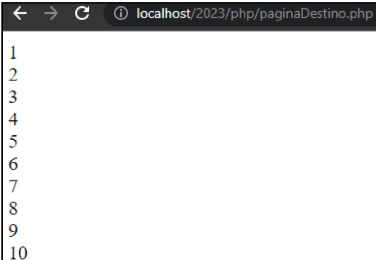
A screenshot of a web browser window. The address bar shows the URL 'localhost/2023/php/paginaDestino.php'. The main content area displays the numbers 1 through 10, each on a new line, representing the output of a PHP do-while loop.
